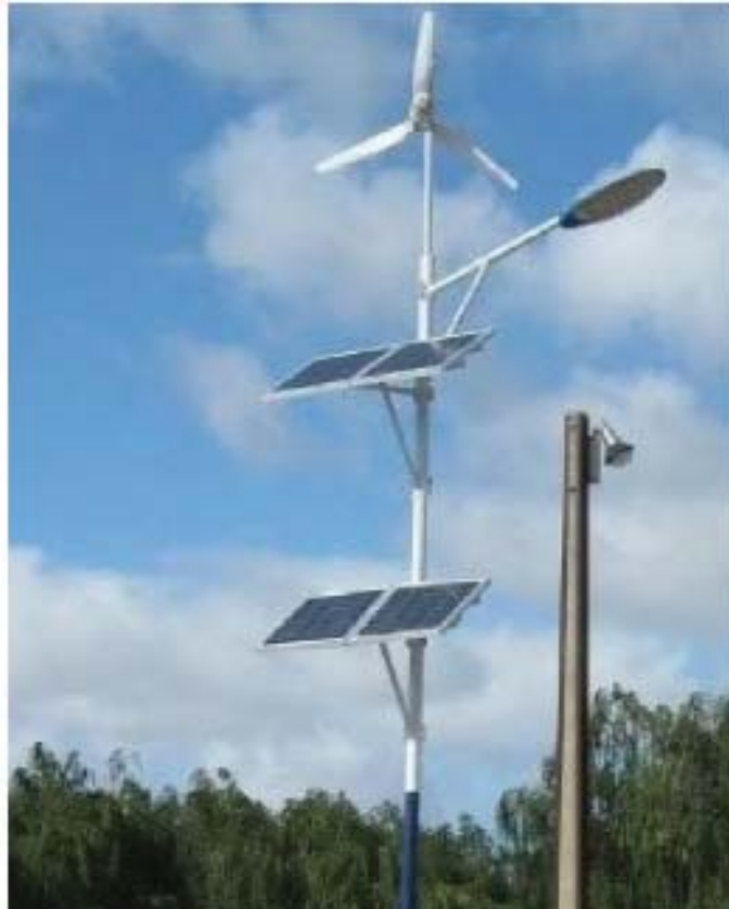
Figure 3: Hybrid System Concept - A wind turbine upon which are placed supplementary solar (PV) panels. It is hoped that the integration of the two renewable energy sources can help maximise the power output of a domestic-size, and improve the system's economics.
