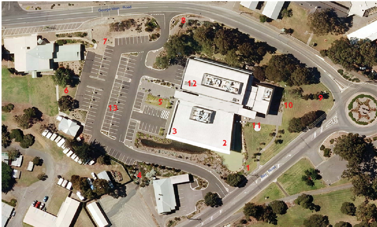
Figure 25: System siting selection. Possible locations at the Civic Centre. Note Sites 1 & 8 were deemed unfeasible due to power lines.
