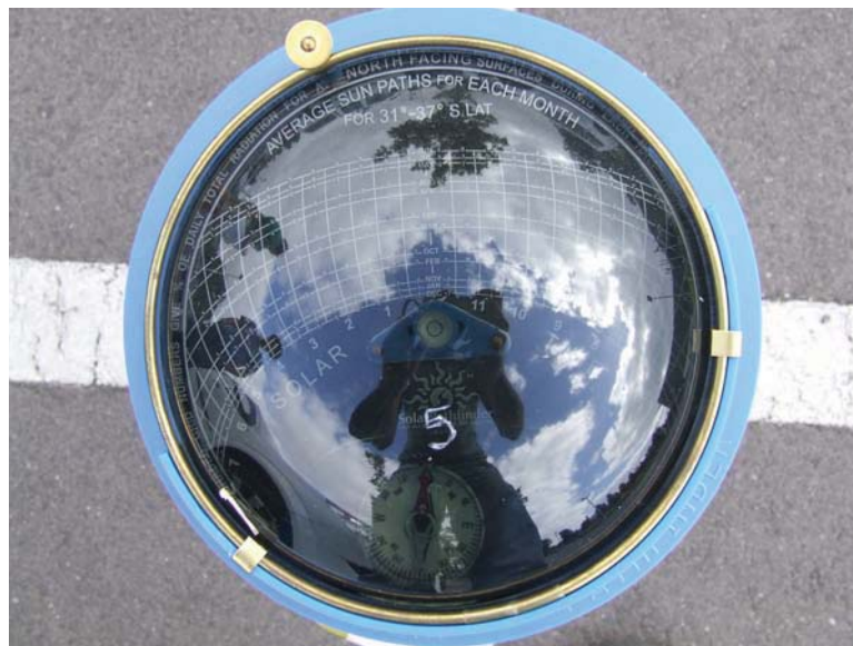
Figure 20: A Solar Pathfinder system that can be used to assess shading effects at PV possible installation sites.
